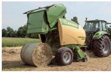
a rotor cutter with 17 or 26 blades and also twine or net wrapping, a single or tandem axle and choose among various operator control units.
