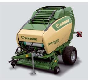
set to handle all crops and conditions. Smaller bale sizes are often preferred in grass silage whereas larger bales are more typical in hay and straw. It is also possible to choose a softer core, which is useful in hay, for example, as it allows moisture to evaporate from the bale.
